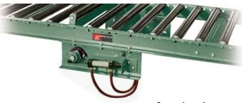
Pneumatic gravity conveyor stops are used where automatic line control is required such as slug accumulation, indexing, etc. This stop is designed for 3-1/2" and 4" deep frames.
