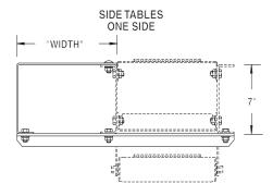
Side tables are commonly used by workers in assembly operations when mounted on roller bed, slider bed and boxed slider bed belt conveyors.
